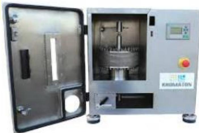
Fig. 9: Sample injector
