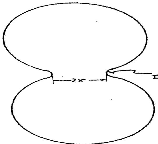
**Fig. 1: Two-sphere sintering model, showing the diameter (2 x) of the neck between the particles and the radius (r) at the end of the neck [1]**
