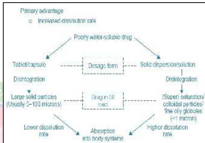
Fig. no.3: Advantages of a solid dispersion formulation, as compared to conventional capsule or tablet formulations
